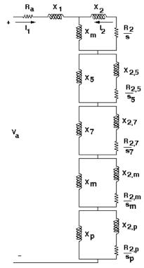
Figure 2: Extended Equivalent Circuit
