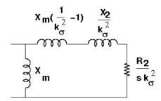
Figure 3: Rotor Section modified by Skew
