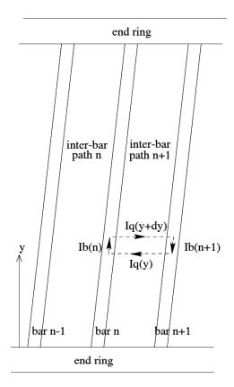
Figure 4: Illustration of skewed rotor bars<sup>5</sup>
