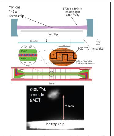
(top) Ion trap chip and resonator, showing details of the trap electrodes. (bottom) photograph of MOT above ion trap chip, with 300,000 atoms.
