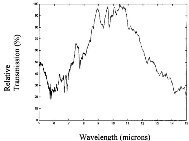
Fig. 4. Transmission through the hollow waveguide around a  $90^\circ$  bend as a function of wavelength.
