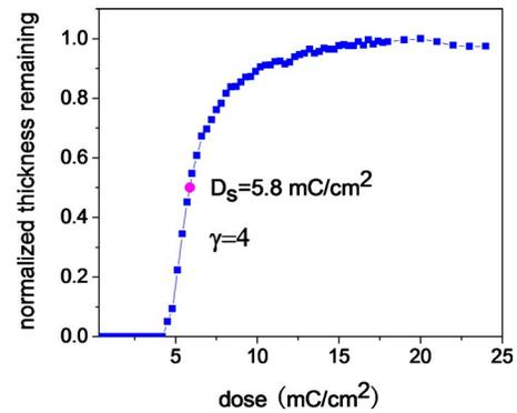
FIG. 3. (Color online) Plot of normalized thickness remaining of PMMA film as a function of dose using MIBK as the developer at 30 °C for 2 min. The contrast value  $\gamma$  and sensitivity  $D_s$  were  $\sim 4$  and 5.8 mC/cm<sup>2</sup>, respectively. It should be noted that the minimum area dose we used in the exposure was 300  $\mu\text{C}/\text{cm}^2$ , so the positive-tone behavior of PMMA was not shown in this figure.
