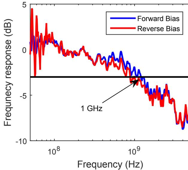
Fig. 8. The 3 dB bandwidth under both forward and reverse bias is around 1 GHz
